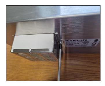
3. Fit and fully tighten the security screws on both sides.
