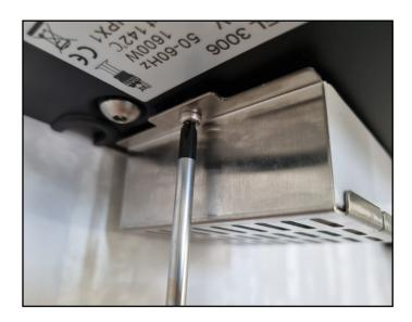
3. Fit and fully tighten the security screws on both sides.
